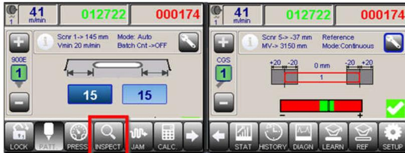
Figure 91: Navigating to the Inspection Window
