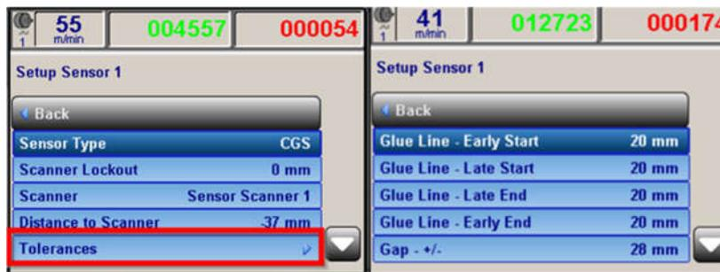
Figure 93: Inspection Channel's Tolerance Menu
