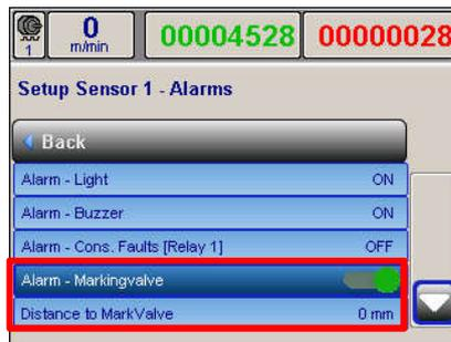
Figure 57: Marking Valve Enable
