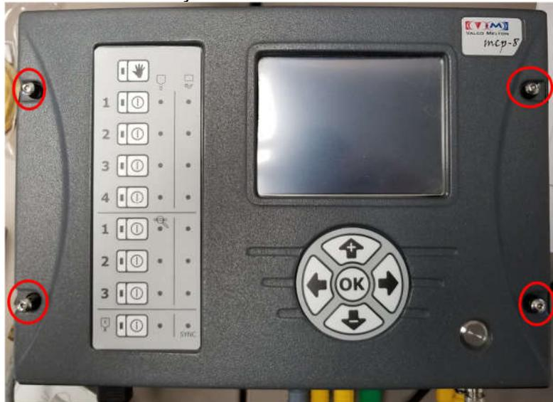
Figure 1: MCP8I Overlay Screw Locations
