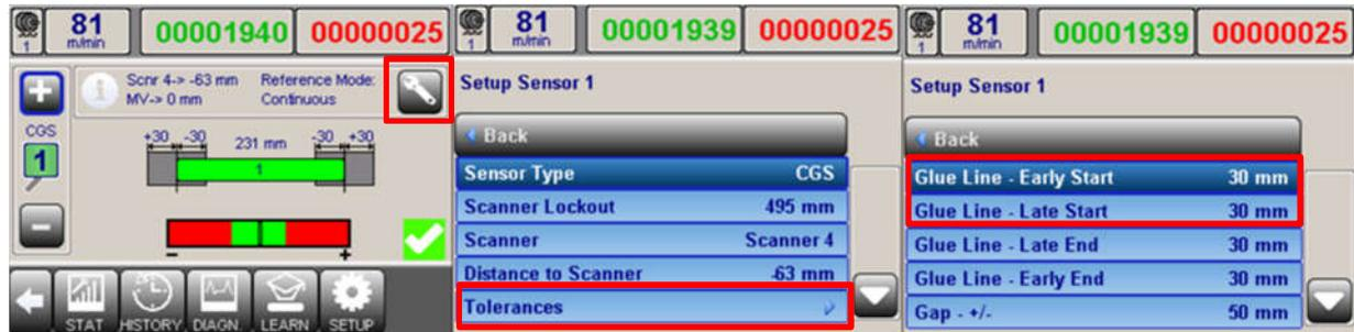
Figure 34: Glue Line Start Tolerances Navigation
