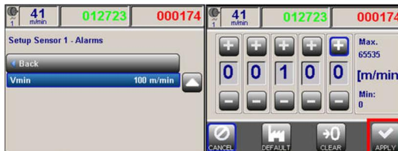
Figure 118: Setting the Sensor Channel's Vmin Setting
