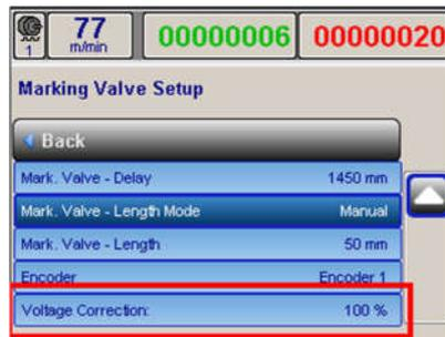
Figure 63: Marking Valve Voltage Correction
