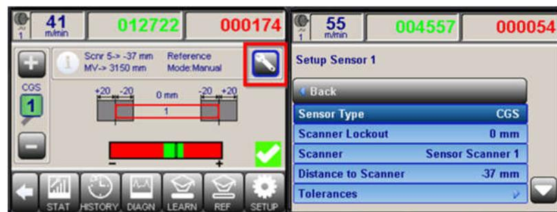
Figure 113: Navigating to the Sensor Channel's Settings
