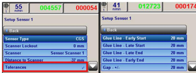
Figure 77: Inspection Channel's Tolerance Menu
