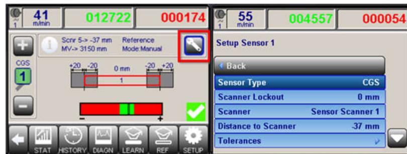
Figure 110: Navigating to the Sensor Channel's Settings
