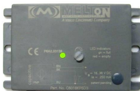
Green Light → Full; Output not activated
